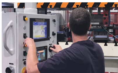
A 10,000-lb.-capacity feedline with coil car allows one coil to run while another is changed in minutes, above. Step-feed mode reduces die prove-out and setup time, left.
